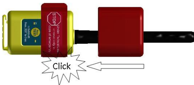
Figure 7: Adding the floating device
