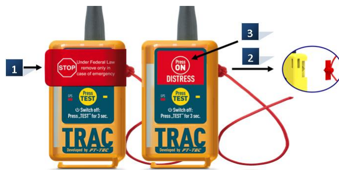
Figure 2: Activating the tracking signal using the ripcord
